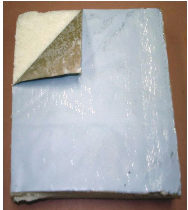
Figure 8a. Foam insulation with cardboard barrier.
